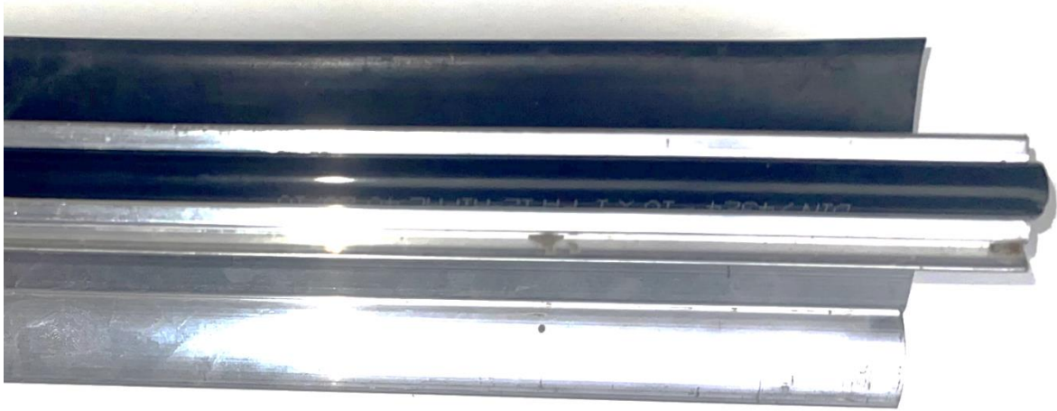
Figure 20 Nylon hose for protecting the support wires
