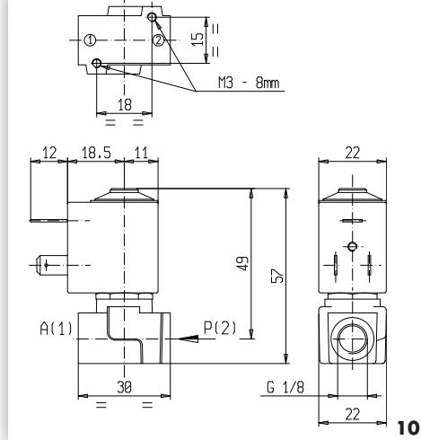
2/2 NC (NORMALLY CLOSED) SOLENOID VALVES PILOT OPERATED - 2/2-WEGE-VENTILE NC (STROMLOS GEZOEGTEN) VORGESTEUERT
