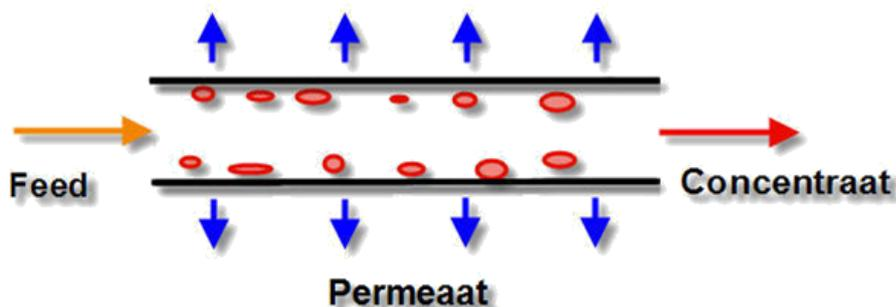
The raw water (feed) is pumped into the pressure cylinders and along the surface of a membrane by the system pump. After these pressure cylinders, the water flow is constricted by means of a needle control valve, which raises the pressure in the cylinders. At this increased pressure, permeate is produced by the membranes. The ratio of permeate to raw water is called the “recovery rate”.
