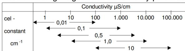
The cell constant must be programmed in step 2.1. You can also set the minimum and maximum limit value with a programmable delay time. In step 9.1 you can set whether the alarm relay must be activated with the relevant message. You can compensate the conductivity measurement for temperature. The water temperature must be programmed in step 3.
