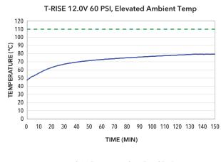
—— Casing Temp — — Casing Temp @ Trip Point
