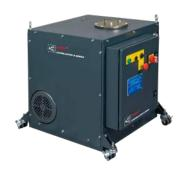
Chipblaster B-30/35 is a single M code controlled, fixed rate medium pressure coolant system. A single pleated, 10-micron filter, automatic overload system, and dirty filter alarm circuit provide a safe machining process that helps prevent damage to the machine-tool, workpiece and tooling. Ideal for machine-tools up to 15 kW (20 hp) and 40 taper mills. The built-in casters make it easy to move for maintenance.
