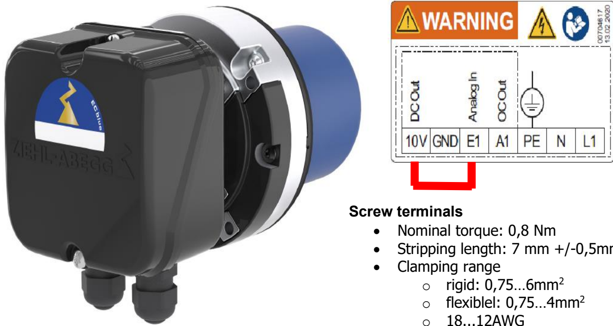
Figure 8 Wiring scheme FG035 fan
