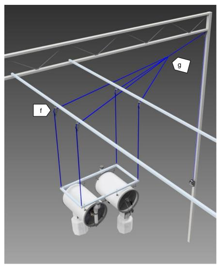
Picture 2 Example of the pulley suspension
