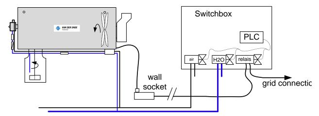
Figure 4 Installation of the Enbar, U2 type
