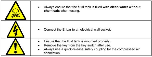
Table 5 Safety regulations for testing the installation
