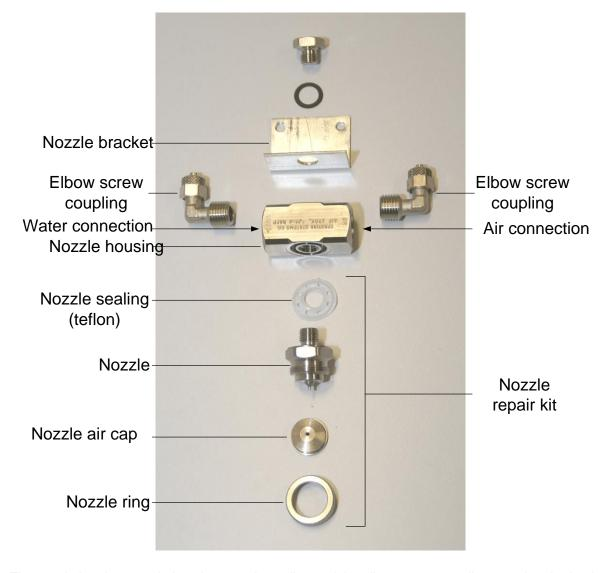
The nozzle bracket, nozzle housing, nozzle sealing and the elbow screw couplings can be obtained separately from the manufacturer. The nozzle sealing, nozzle, nozzle air cap and nozzle ring can be obtained as a repair kit. With the exception of the nozzle sealing, these components cannot be obtained separately.
