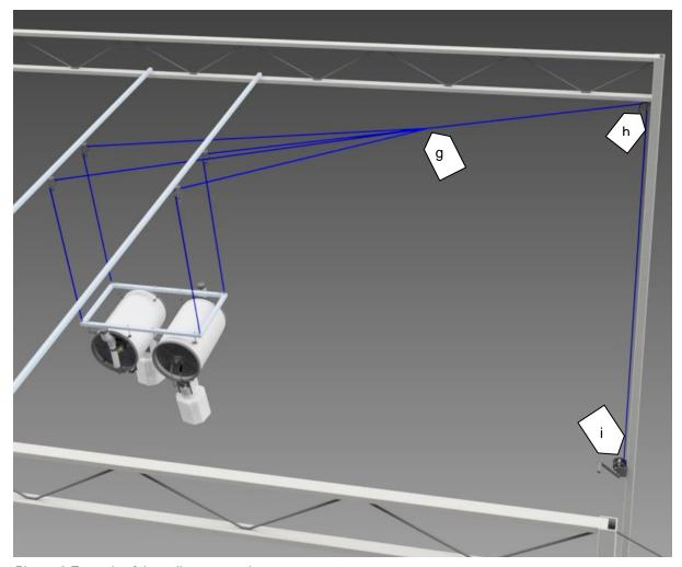
Picture 3 Example of the pulley suspension
