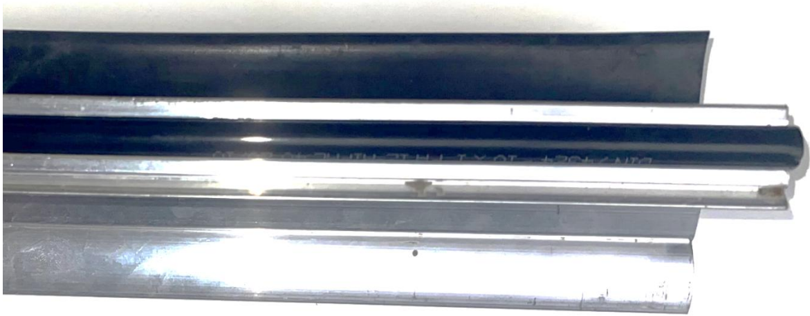
Figure 20 Nylon hose for protecting the support wires
