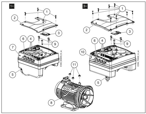
Figure 6: Main components - Single-phase and three-phase models
