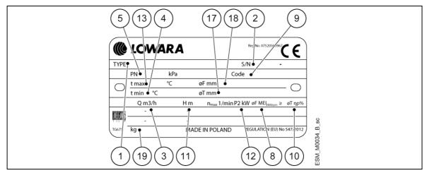
Figure 4: e-LNEEE/e-LNESE/e-LNTEE/e-LNTSE data plate
