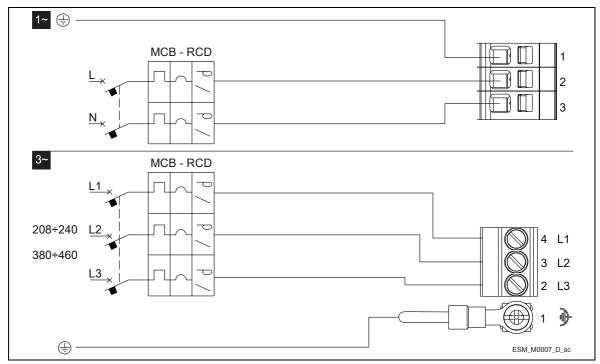
Figure 9: Wiring diagram
