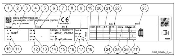
Figure 2: Motor data plate
