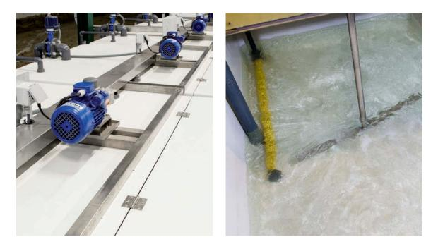
The Enmix Light was specially developed for smaller mixing tanks that can hold up to a maximum of  $2 \text{ m}^3$ .
