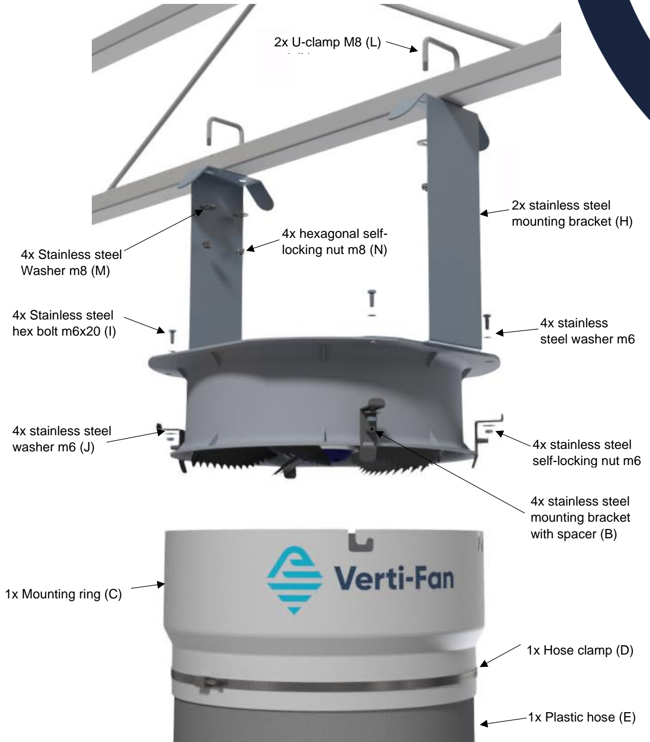
Figure 3 Lowered installation of the Verti-Fan using lowered brackets
