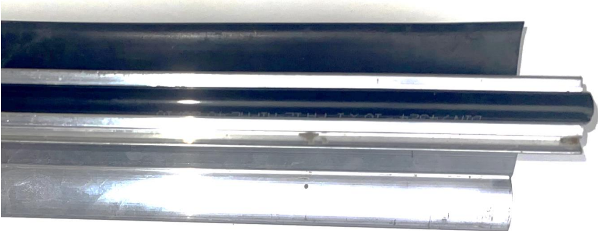
Figure 20 Nylon hose for protecting the support wires
